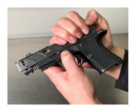
2. Remove recoil spring assembly. NOTE: Compensator cannot be removed while recoil spring assembly is installed.
