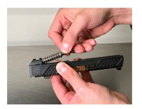
3. Familiarize yourself with the location of the detent by pushing the barrel forward in the slide and viewing the rear of the compensator. You will note that inserting the disassembly tool into the Side Access Slot will allow you to depress the plunger with the SIDE of the tool.
